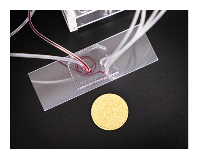
A close-up of the lab-on-a-chip prototype (compared to a SGD \$1 coin) developed by the NTU Singapore, Tan Tock Seng Hospital and MIT, which can extract extracellular vesicles (EVs) in a one-stop process. The amount of EVs can indicate if a diabetes patient is having vascular inflammation. Credit: Nanyang Technological University
