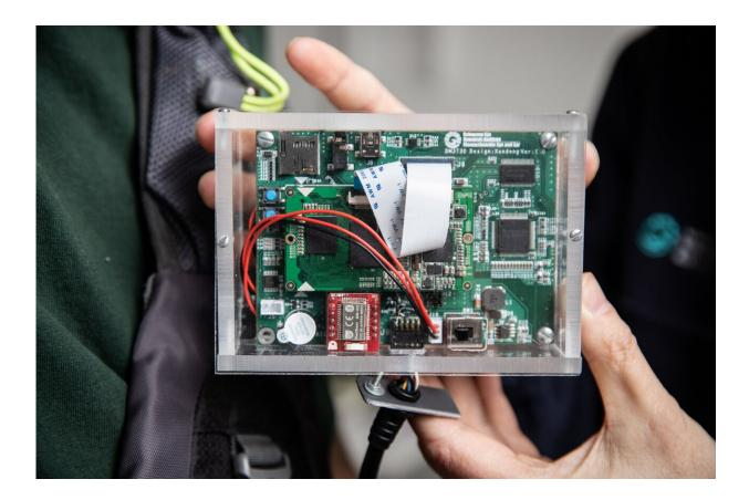
A close-up of the image processing unit of the wearable collision device. Credit: Mass Eye and Ear
