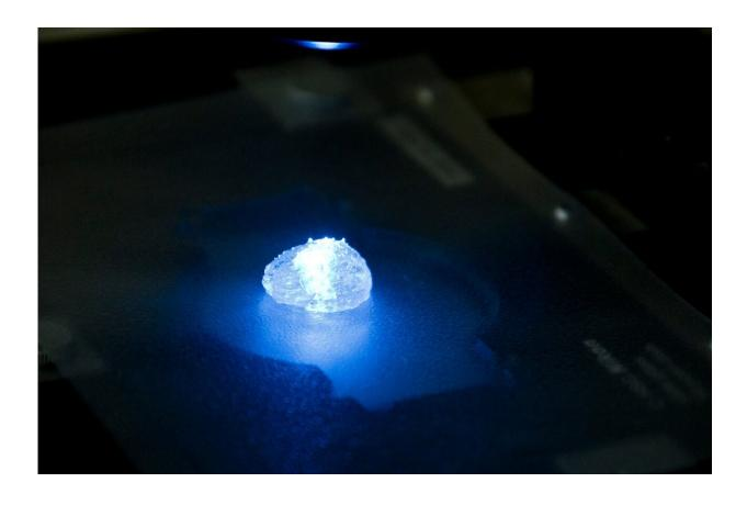
Demonstration of 3D printing of a tumor in a brain Microenvironment according to a computed 3D model. Credit: Tel Aviv University
