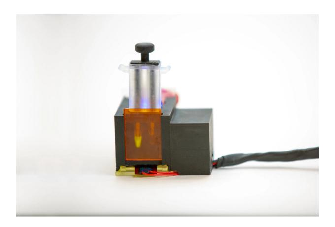
miSHERLOCK is a self-contained at-home diagnostic platform that allows users to test their own saliva for the presence of SARS-CoV-2 and can distinguish between multiple variants of the virus. Credit: Wyss Institute at Harvard University
