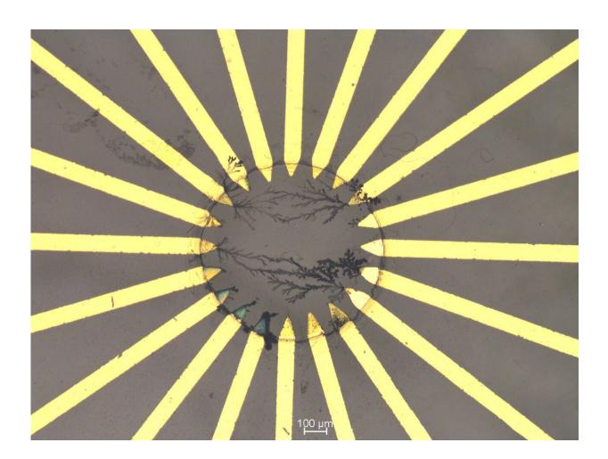
Artificial polymer-based neural network. The strongly nonlinear behavior of these networks enables their use in reservoir computing. Credit: TUD
