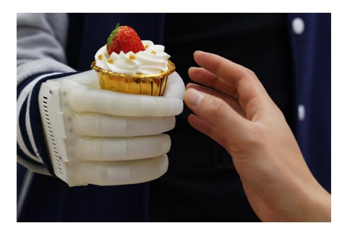
Caption:An MIT-developed inflatable robotic hand gives amputees real-time tactile control. The smart hand is soft and elastic, weighs about half a pound, and costs a fraction of comparable prosthetics. Credit: Massachusetts Institute of Technology
