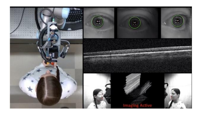
Duke's newly developed OCT scanner is attached to a robotic arm that can move the scanner to perfectly align with a patient's eyes. The scanner requires less than 10 seconds to scan and image each eye. Credit: Duke University
