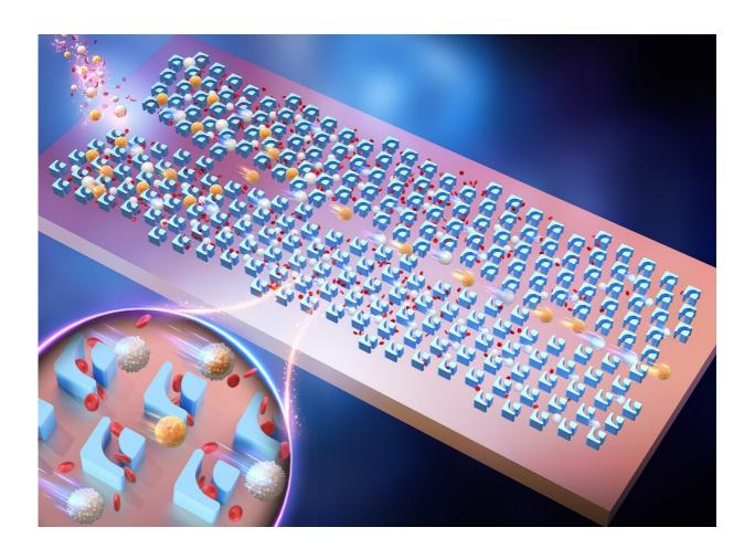
Fig 1. Cascaded filter deterministic lateral displacement microfluidic chip. Credit: SIAT
