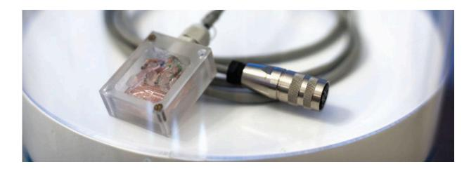
MEG-feasible fluxgate magnetometer. Credit: Maxim Ostras/RQC
