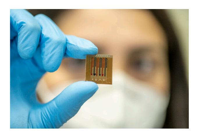
The microfluidic multiplex biosensor carries proteins attached to a polymer film that recognize the antibiotics. Credit: Patrick Seeger
