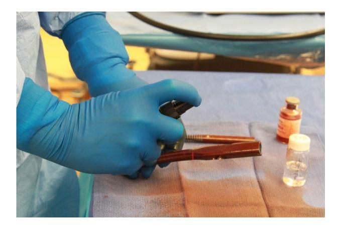
After mixing self-assembling polymers with antibiotics, the infection-preventing coating is sprayed on to human intramedullary hip implants with a simple perfume bottle. Credit: Duke University
