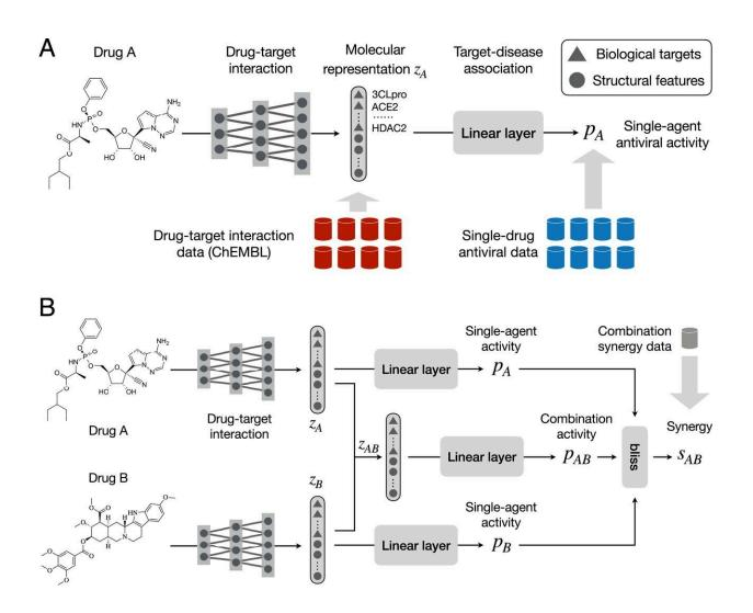
ComboNet for synergistic drug combination discovery. (A) ComboNet is composed of two networks: a DTI and a target–disease association network. The antiviral effect of a single drug pApA is predicted from its representation zAzA. The vector zAzA characterizes the DTI features of drug A. (B) The antiviral
