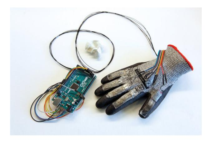
The sensor material used in the glove is extracted from naturally available silk cocoons. The glove itself consists of five channels, each one attached to one of the five fingers of the hand. Whenever a sensor is deformed a resistance change occurs, which subsequently is converted and transmitted to a computer via an Arduino board. Credit: Jesper Scheel
