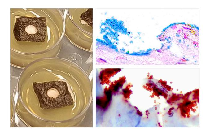
The equine ex vivo skin biofilm explant model with an image of skin explants in culture (left) and bacterial biofilms stained with Alcian Blue (upper right) and an anti-bacterial antibody (lower right) to show the presence of bacteria in the skin biofilm explant model. Credit: AlphaMed Press
