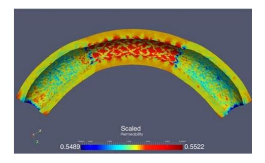
Permeability of the arterial wall with an implanted stent. Blue represents regions of low permeability and red represents regions of high permeability. There is high permeability between the stent struts but low permeability near the stent edges. The mostly rigid stent does not allow the nearby arterial tissue to freely expand, leading to tissue compression. Credit: Sunčica Čanić, Yifan Wang, and Martina Bukač
