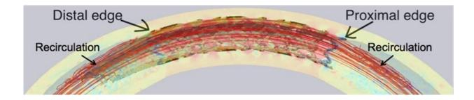
Several streamlines of blood flow inside the stented artery. Recirculation zones are present near the edges of the stent, where the blood does not flow down the artery normally. Credit: Sunčica Čanić, Yifan Wang, and Martina Bukač
