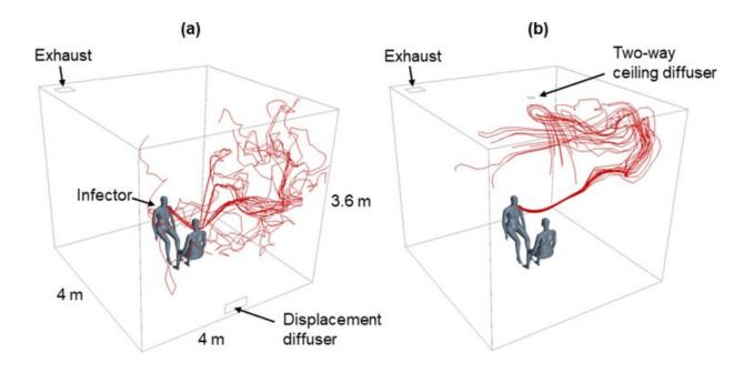
Displacement ventilation (left), used in most homes, can increase the rate of transmission of aerosols from one person to another seven times quicker than mixed-mode ventilation (right), which is found in many commercial buildings. Credit: Donghyun Rim/Penn State
