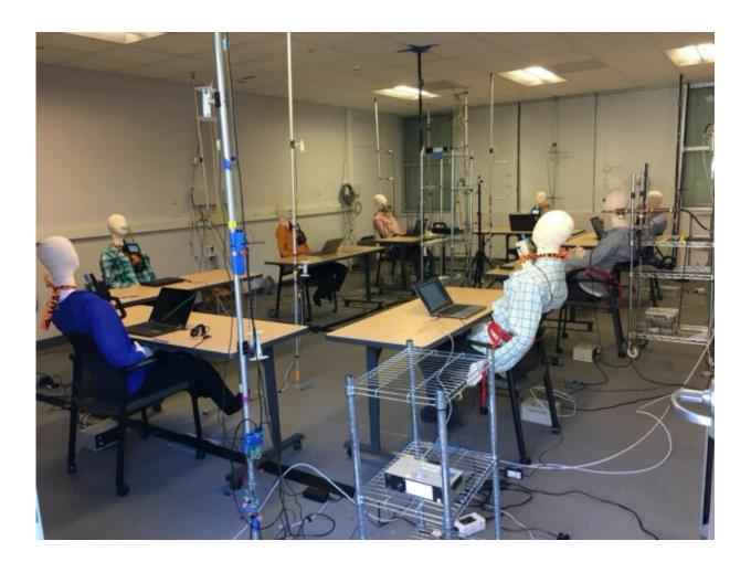
In one of the room configurations, Berkeley Lab researchers put eight participants facing inward like in a meeting. One manikin, designated as the "speaker," was outfitted with a device to expel aerosols to simulate a person talking. The other manikins had a CO2 sensor and optical particle counter placed in their breathing zone. There were also sensors throughout the room to measure temperature, air velocity, and CO2. Credit: Lawrence Berkeley National
