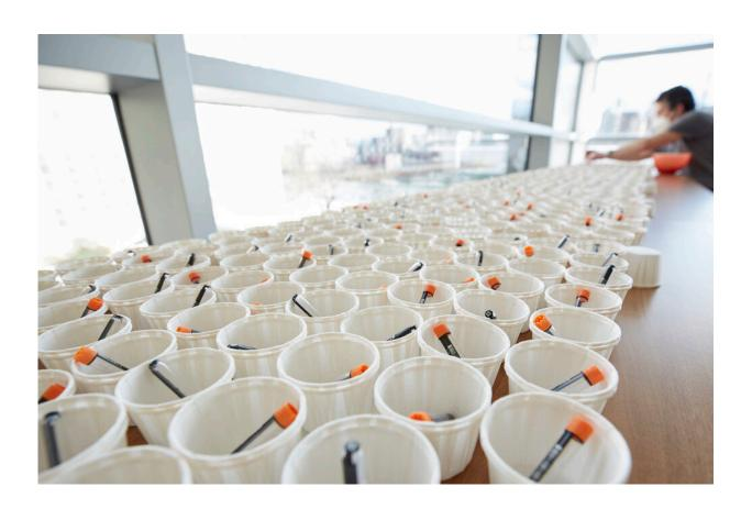
Stored in orange-capped vials for mass distribution, the DRUL buffer is part of an inexpensive saliva-based COVID test developed at Rockefeller. Credit: Rockefeller University
