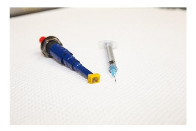
Georgia Tech's ePatch, containing a microneedle electrode array (yellow) affixed to an electroporation pulser made from a BBQ lighter (blue), is shown next to a needle and syringe. Credit: Candler Hobbs, Georgia Tech
