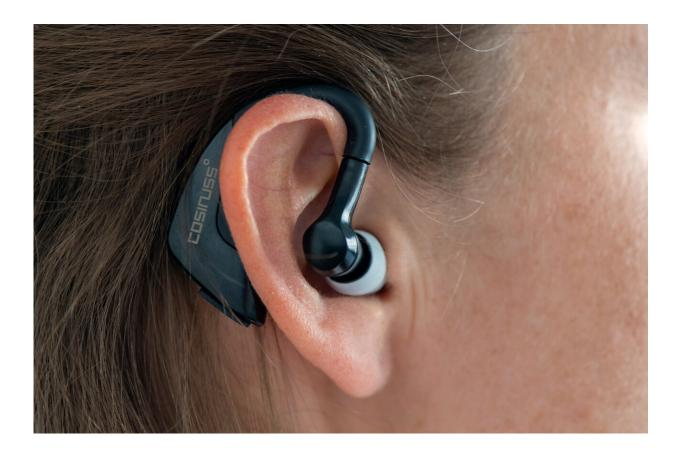
The ear sensor is to be worn behind the ear like a hearing aid. It transmits the most important vital parameters every 15 minutes. If the values worsen, the patient is contacted and, if necessary, admitted to the hospital. Credit: Andreas Heddergott / TUM
