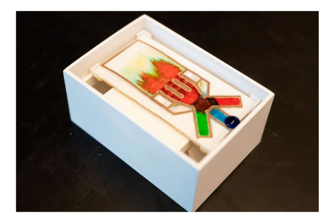
This is the fully assembled liquid flow assay developed in the Sarioglu lab. Credit: Allison Carter
