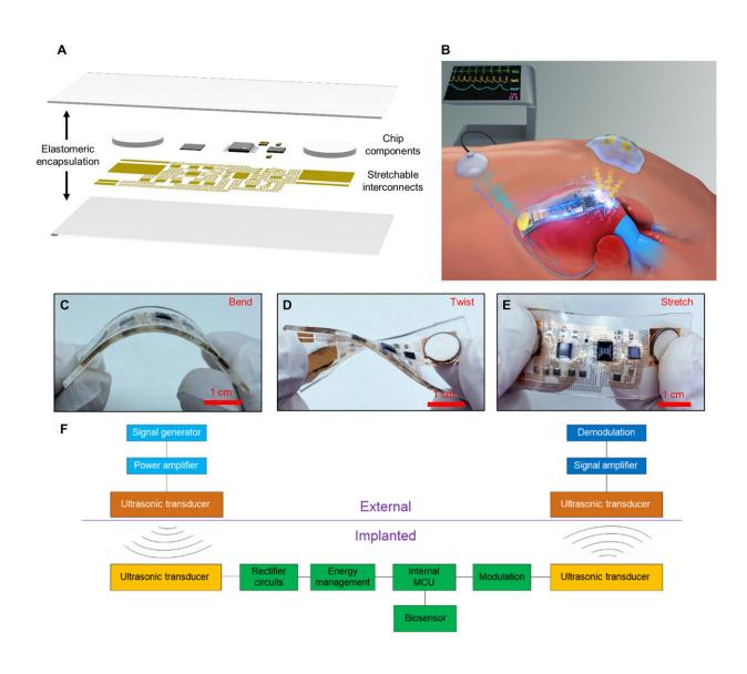
Schematic illustration of the AECD. (A) Exploded schematics of the device
