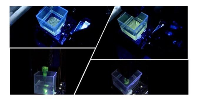
The fabrication process of a biomimetic cochlea: creating an electro-mimetic bone matrix (top images) and a spiral-shaped cochlear structure within the matrix (bottom images). Credit: Iek Man Lei
