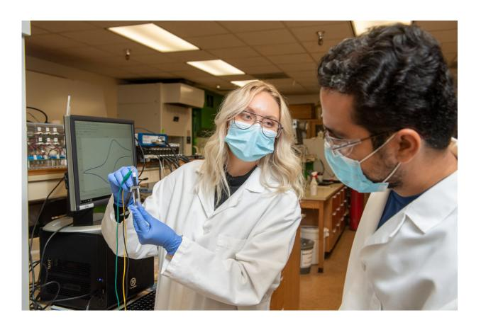
Postdoctoral researcher Abdelrhman Mohamed and graduate student Gretchen Tibbitts used an electric probe to measure bacterial electrochemical signals and to identify antibiotic resistance in less than 90 minutes. Credit: WSU
