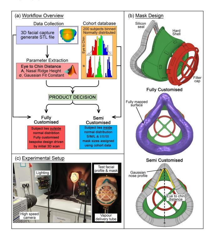
Figure 1. (a) Workflow from scan to product, (b) mask design highlighting fully customized and semi-customized aspects, (c) experimental setup for flow visualization used to rapidly assess fit. Credit: DOI: 10.1038/s41598-021-00341-3
