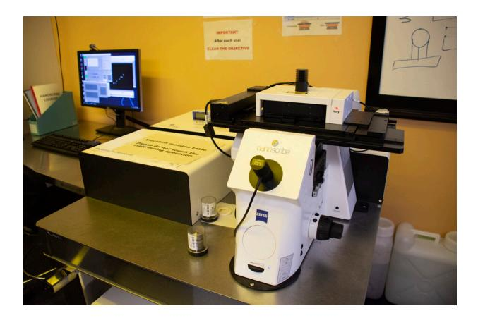
The Nanoscribe printing machine uses 2-photon lithography to print and then harden polymer to form specifically designed structures. Credit: Okinawa Institute of Science and Technology
