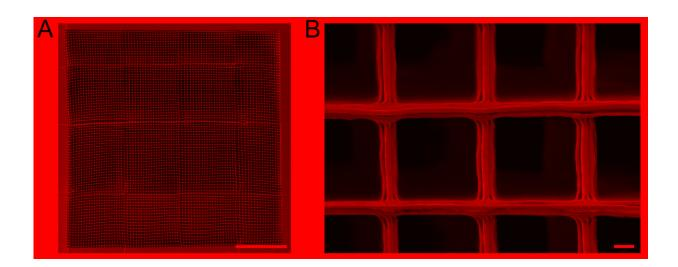
The scaffold, imaged using an electron microscope, is structurally designed to help guide regenerating neurons. Image A: scale bar =  $100 \mu m$ . Image B: scalebar =  $1 \mu m$ . Credit: Okinawa Institute of Science and Technology
