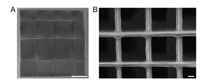
The scaffold, imaged using an electron microscope, is structurally designed to help guide regenerating neurons. Image A: scale bar =  $100 \mu m$ . Image B: scalebar =  $1 \mu m$ . Credit: Okinawa Institute of Science and Technology
