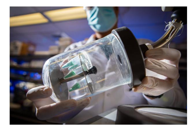
A vacuum chamber holds ingredients of a liposome-based vaccine that could be developed for COVID-19. The chamber is used for freeze-drying products. Credit: Douglas Levere / University at Buffalo
