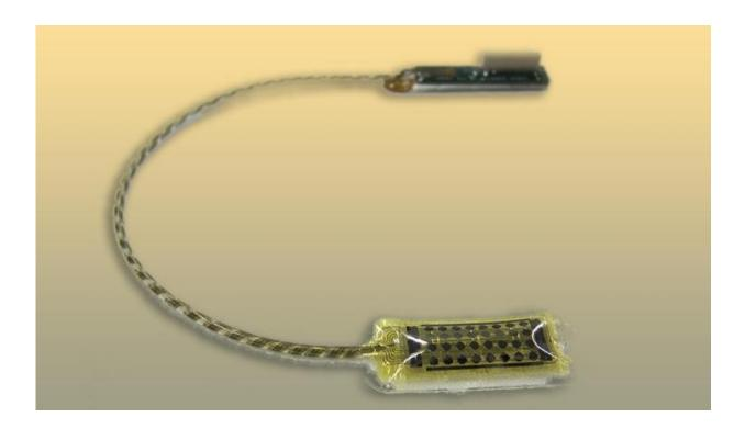
In a recent study by a Lawrence Livermore National Laboratory (LLNL) and University of California, San Francisco team, researchers found that the flexibility of LLNL-developed thin-film microelectrodes, combined with higherdensity grid spacing, provides greater levels of detail about how the brain works, while also providing the ability to stimulate areas of the brain affected by epilepsy and other neurological disorders. Credit: Lawrence Livermore National Laboratory
