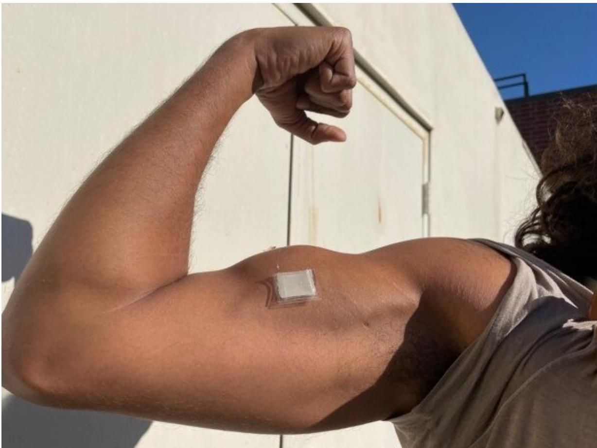
Scientists have developed improved methods to fabricate epidermis-inspired pressure sensors. These sensors have wide-ranging sensitivity to body movements, from joint and muscle flexing to minute pulse rates. Credit: Terasaki Institute for Biomedical Innovation
