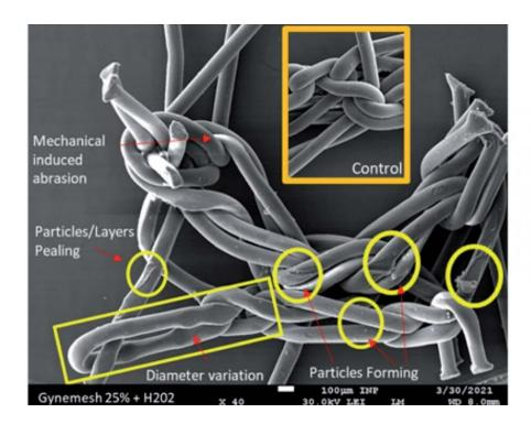
PP mesh—the cause of the vaginal mesh scandal—before and after being tested using the new method. The test shows that the PP mesh starts to crack after being tested in conditions similar to inside the human body. Credit: University of Sheffield
