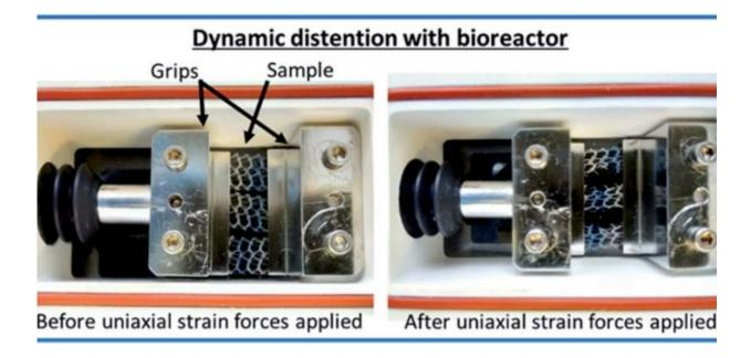
PP mesh before and after being stretched and put under pressure within a bioreactor—this is part of the new test that enables materials to be tested in conditions similar to inside the human body. Credit: University of Sheffield
