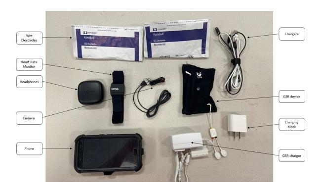
The components of the Bio Ware kit. Photograph provided by Periscope. Credit: Zeriscope.
