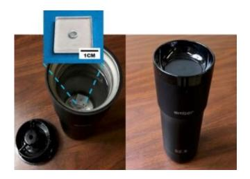
Photographs of commercially available, battery-operated coffee mug used as a water bath for isothermal amplification. (left) Coffee mug is open, containing detection units in a water bath. A picture of the detection unit is shown in the inset above the mug. (right) Coffee mug is closed during RT-LAMP amplification at 62.5 degrees C. Credit: University of Florida
