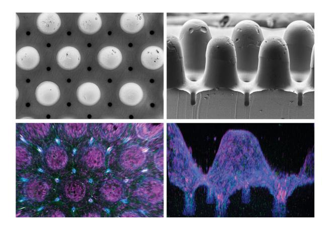
Bioengineered organoids with an in vivo—like tissue architecture. Top row: Scanning electron microscopy images of a polymer template used for fabricating hydrogel substrates with a realistic crypt-villus architecture (top and side views, respectively). Bottom row: 3D reconstruction of immunofluorescence images showing an intestinal tissue with realistic crypt and villi — "peaks and valleys" — anatomy of the real organ. Credit: Mike Nikolaev (EPFL)
