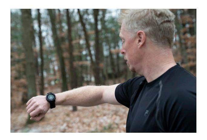
Lincoln Laboratory researcher James Balcius tests the heat strain detection device. The smartwatch displays a thumbs-up and green background, indicating that he is not at risk of heat injury at this time. Credit: Glen Cooper
