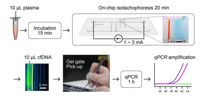
Scientists from Shibaura Institute of Technology (SIT) designed an open-channel microfluidic gated device to purify and separate short fragments of pathogenic DNA such as the MTB genome from human plasma samples. Credit: Nobuyuki Futai from SIT, Japan
