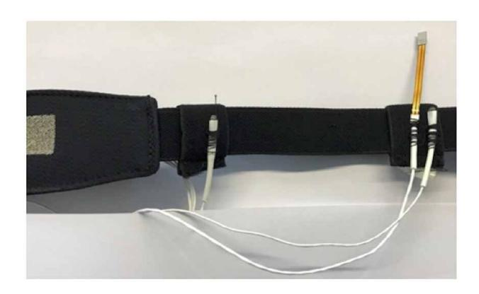
Figure 1. Skin temperature sensors (white) and heat flux sensor (orange) attached to the ECG belt. Notes: ECG and heat flux data were not analyzed in this study but were considered for another aspect of the project. ECG, electrocardiogram. Credit: DOI: 10.3389/fnagi.2021.585904
