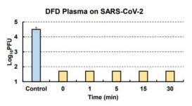
Experiment of real time coronavirus inactivation through joint research between KIMS and Masan National Tuberculosis Hospital (PFU decreasing tendency by accumulated time after passing through plasma filter). Credit: Korea Institute of Materials Science (KIMS)
