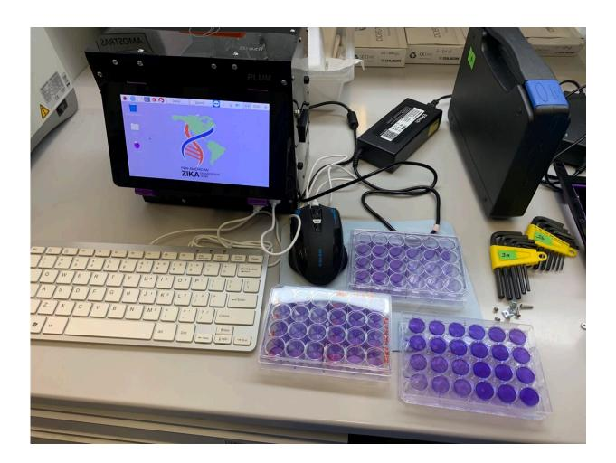
A "lab-in-a-box", the PLUM reader (Portable, Low-cost, User-friendly, Multimode), presents results from up to 384 patient samples and displays them in a single image capture. PLUM is also highly programmable and can be similarly applied to detect any pathogen sequence. Credit: Livia Guo, LSK Technologies
