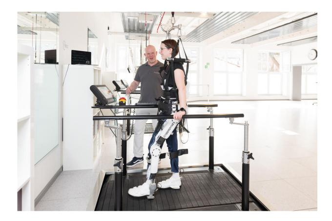
The Hybrid Assistive Limb (HAL; CYBERDYNE Inc., Japan) is the world's first cyborg-type wearable robot that supports gait training based on the wearer's intended motion. Credit: CYBERDYNE Inc.
