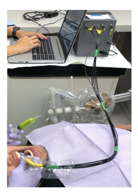
The UW optical O-pH prototype can non-invasively measure the acidity of oral biofilm. Credit: University of Washington and IEEE Xplore/Creative Commons
