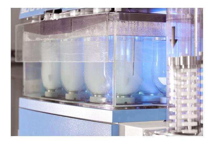
This photo provided by Pfizer shows a test to check if Paxlovid tablets dissolve within a specific amount of time, before the fluid is tested to ensure the proper quantity of ingredients, in Freiburg, Germany in December 2021. Studies showed that the first pill to treat the virus led to a nearly 90% reduction in hospitalizations and deaths among patients most likely to get severe disease. Credit: Pfizer via AP
