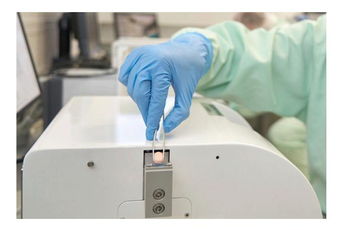
In this photo provided by Pfizer, a lab technician places a Paxlovid tablet into a machine which applies pressure to test the pill's physical strength, in Freiburg, Germany in December 2021. Studies showed that the first pill to treat the virus led to a nearly 90% reduction in hospitalizations and deaths among patients most likely to get severe disease. Credit: Pfizer via AP
