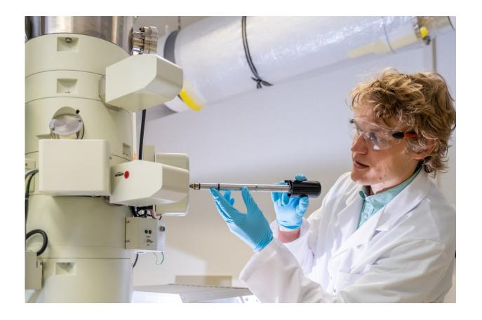
Fire and Ice: Empa researcher Lukas Gerken produces nanoparticles for cancer therapy using flame synthesis. To make the tiny metal particles visible, the electron microscope is cooled to freezing temperatures with liquid nitrogen. Credit: Empa
