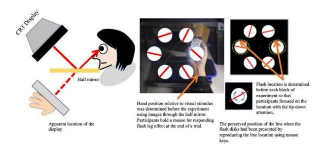
(Left) Experimental set up. Visual stimuli were observed through a half mirror to investigate the effect of an invisible hand, the location of which is identified by proprioception, on the visual processing. (Right? Stimulus conditions and method to measure flash lag effect (FLE). Credit: Satoshi Shioiri
