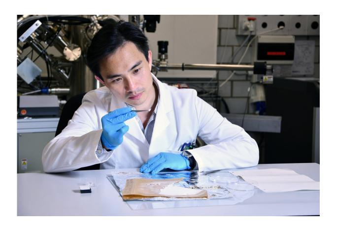
Empa researcher Fei Pan is working on a membrane made of nanofibers that releases medication only when the material heats up. Such a membrane could, for example, become active in a bandage as soon as an inflammation starts. Credit: Empa
