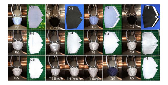
The DREAM Laboratory constructed and tested 12 different face masks using a thermal manikin. Credit: Farzan Gholamreza
