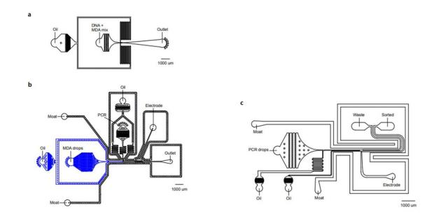
Schematics of microfluidic devices used to: a) encapsulate DNA and MDA reagents into isolated droplets; b) merge MDA droplets with PCR mix droplets; and c) sort individual PCR positive droplets. Credit: Nature Biomedical Engineering (2022). DOI: 10.1038/s41551-022-00864-8
