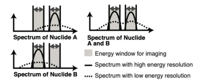
Figure 1: Model explaining the energy resolution. The top left image shows the spectrum of nuclide A, and the bottom left image shows the spectrum of nuclide B. When nuclide A and B are both present, the spectrum looks like the top right image. Imagers with limited energy resolution detect nuclides A and B as a low plateau with two small peaks, but an imaginer with improved energy resolution can detect individual A and B spectra. Credit: Yagishita et al.
