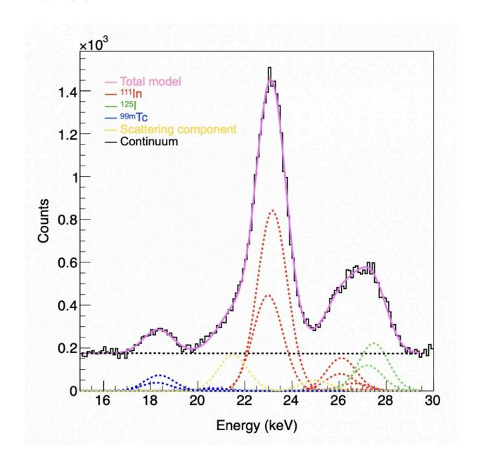
Figure 4b: The total spectrum (black solid line) and the individual spectra (colored dotted lines) identified and separated using the fitting method. The black line indicates the data obtained by the imager. Indium-111 (red), iodine-125 (green), and technetium-99m (blue) spectra were separated from the overall spectrum by fitting. Credit: Yagishita et al./Kavli IPMU
