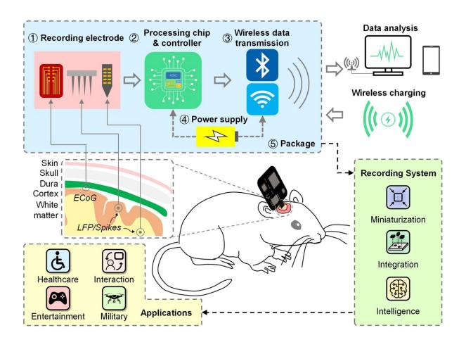
A typical configuration of wireless neuronal recording systems consists of five modules: (1) implantable electrodes for neural signal acquisition; (2) processing chips and controller for signal amplification, filtering, multiplexing, digitization, and controlling the parameter setting; (3) wireless data transmission to computers or other portable equipment for further data analysis; (4) power supply by
