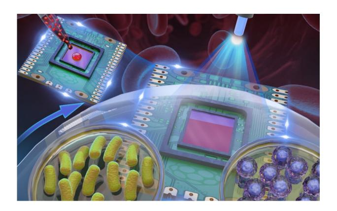
Blu-ray microscope with blood-cell lens. The scheme of the microscope device modified from a Blu-ray disc. A monolayer of blood cells was smeared on top of the image sensor as a high-resolution computational lens with a theoretically unlimited field of view. Credit: Guoan Zheng
