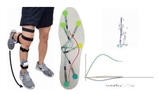
An interdisciplinary team of University of Massachusetts Amherst researchers has developed a low-cost shoe insole, equipped with forcesensitive resistors (FSR), that aims to improve the management of health conditions that impair mobility, such as stroke, Parkinson's disease and osteoarthritis.
